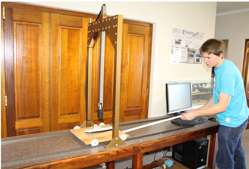
The ship is tested using a magnetic sensor to determine if it has been sufficiently degaussed.
