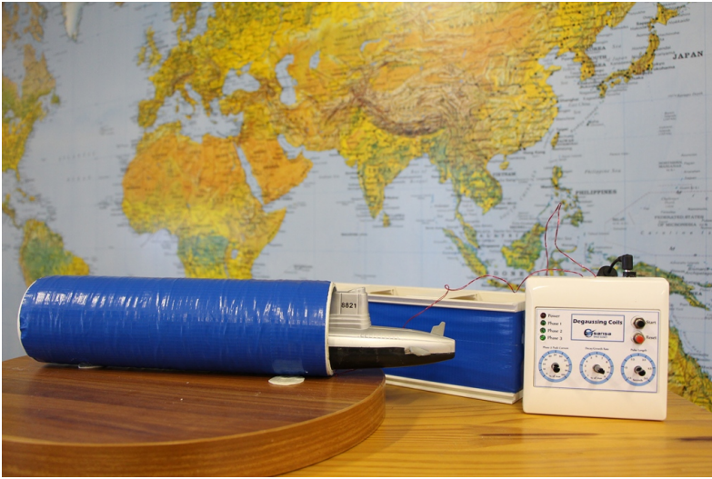
The model ship is placed in the degaussing coil system designed to reduce the magnetic signature of the ship.
