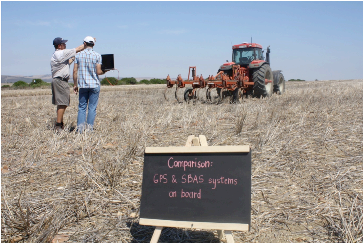
A tractor equipped with both the standard GPS and the SBAS antennas, as well a radio antenna; used to conduct the Precision Farming trials
