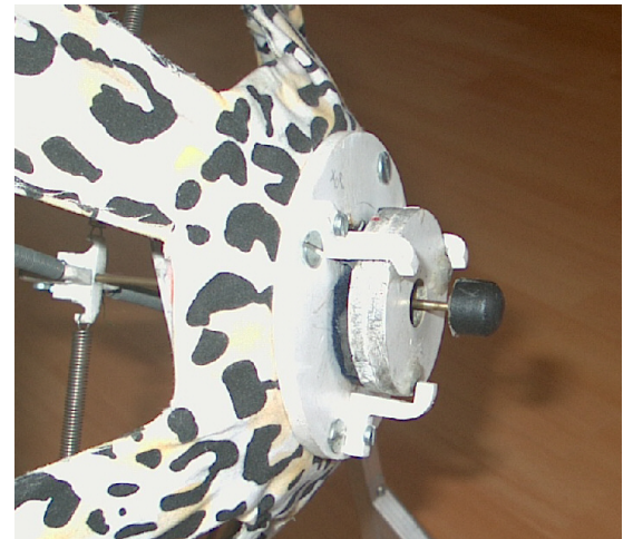
Figure 4 (right): Mute plate on linear generator. A hard or full stroke on the armature tip causes the plate to move in and close one or both micro-switches which sets a mute function. A light stroke causing travel of less than 10 mm does not enable the mute function.
