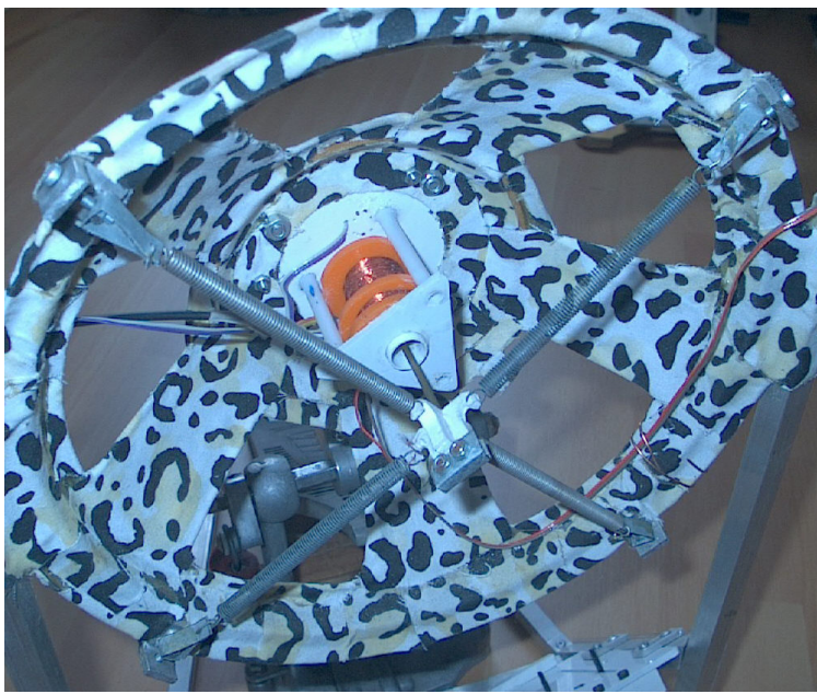
Figure 4 (right): Mute plate on linear generator. A hard or full stroke on the armature tip causes the plate to move in and close one or both micro-switches which sets a mute function. A light stroke causing travel of less than 10 mm does not enable the mute function.
