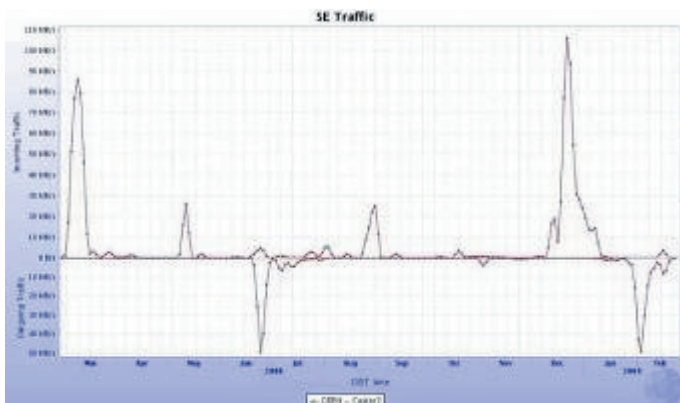
Figure 3: Data rates to and from the ALICE central storage at CERN over the last year. Much of this data is real Physics data from cosmic events.
