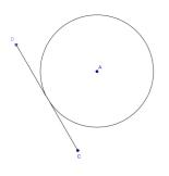
A line segment that touches the circle at only one point (like DC in the accompanying figure) is called a **<u>tangent</u>** to the
