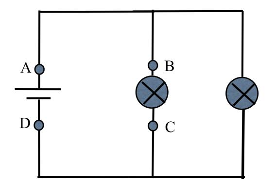
Compare the current through the bulb connected between B and C now to the current through it before when there was only one bulb.
