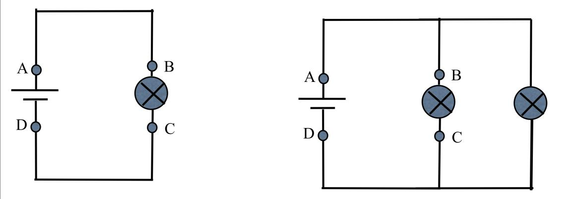
A second identical bulb is added to the circuit on the left, as shown.
