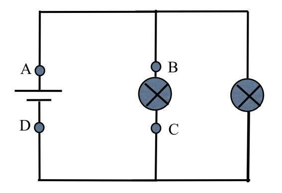
Compare the brightness of the bulb connected between B and C now to its brightness before when there was only one bulb.
