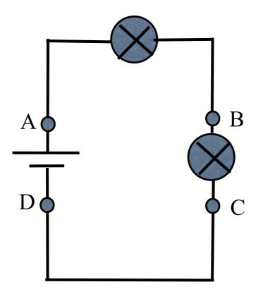
Compare the current through the bulb connected between B and C now to the current through it before when there was only one bulb.
