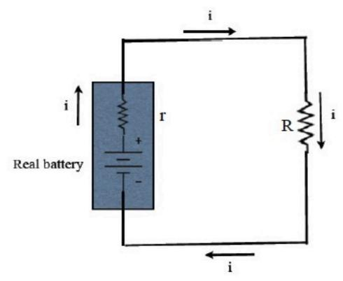
Going around this loop in a clockwise direction, and realising that the voltage decreases through every resistor, we have  $\mathcal{E} - ir - iR = 0$  or  $i = \mathcal{E}/(R + r)$
