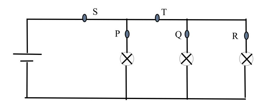
In the circuit shown, all the bulbs are identical. The current at P is 0.2 amps. What are the currents at
