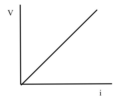
The slope or gradient of this line is the resistance R.
