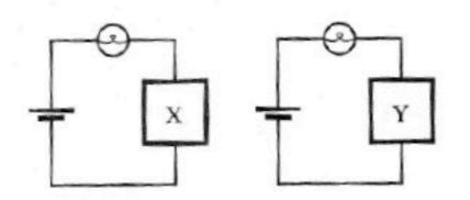
The bulb on the left is brighter than the bulb on the right. Compare the resistance of X with that of Y
