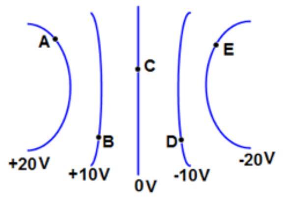
A non-uniform electric field is represented by equipotential lines. What is the direction of the electric field at point A?
