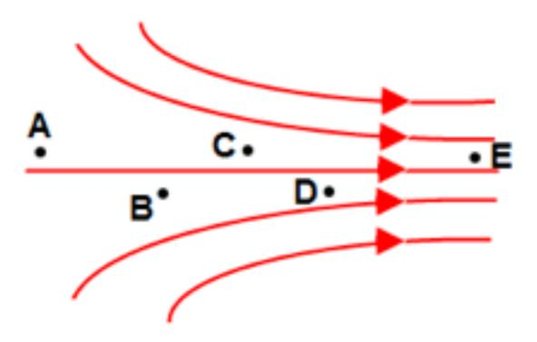
A non-uniform electric field is represented by the diagram. At which of the following points is the electric field greatest in magnitude?
