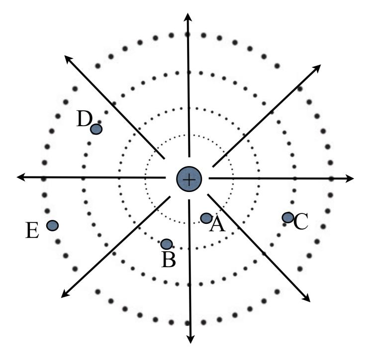
An electric field due to a positive charge is represented by the diagram. Which of the following points has higher potential?
