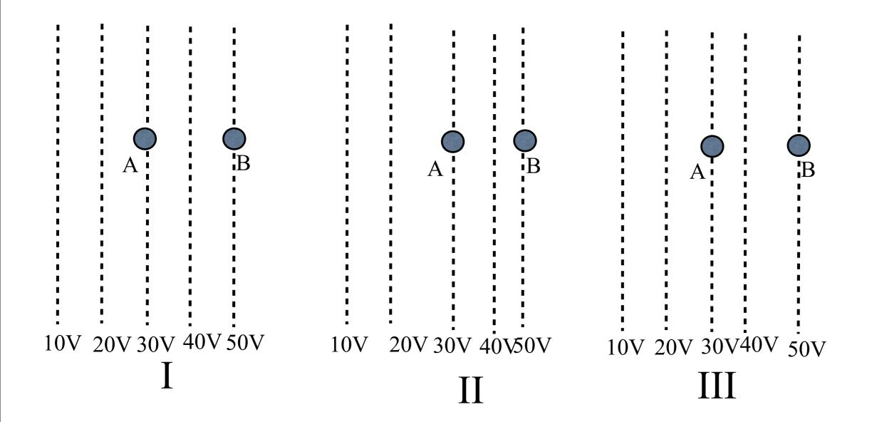
1. The five lines represent values of the potential along those lines. These are called equipotentials. A  $1\mu$ C positive charge is moved from A to B. How does the amount of work needed to move this charge compare for these three cases?
