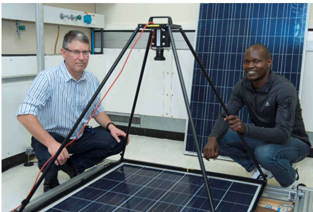
Professor Ernest van Dyk and PhD student Isaac Kwembur inspect electroluminescence equipment used to evaluate PV modules.
